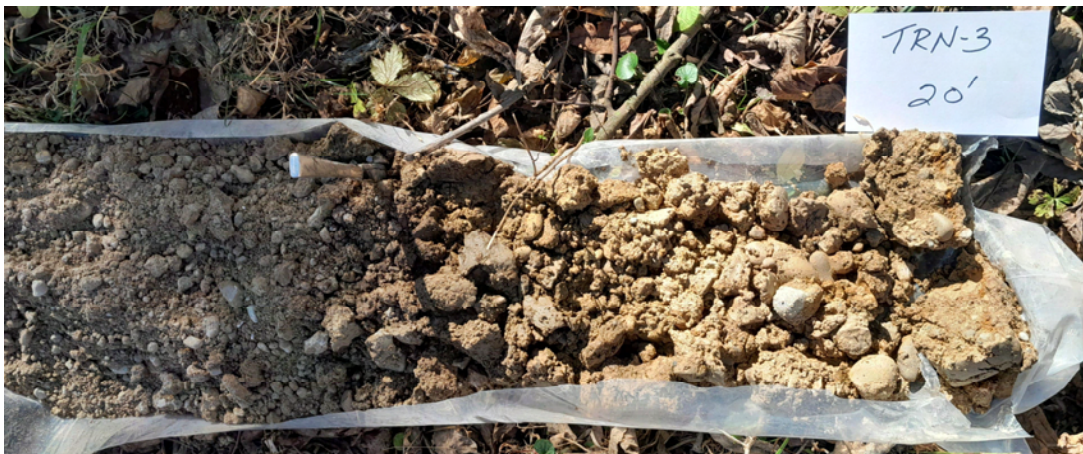
Figure 16. Silty gravel and sand as encountered in TRN-3 from 15 to 20 ft. bgs.
