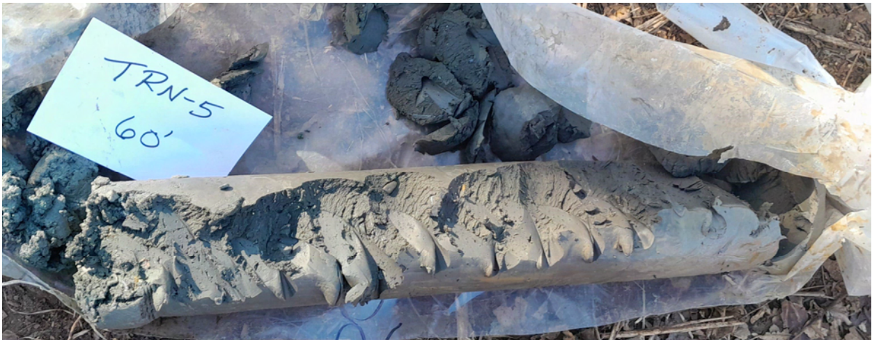
Figure 29. Silty clay glacial till encountered from 58 to 60 ft. bgs at TRN-5.
