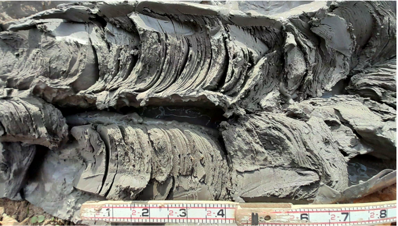
Figure 24. Close up of varved lacustrine clay deposit as encountered from 43 to 70 ft. bgs at TRN-4.
