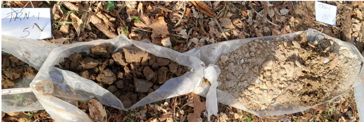
Figure 5. Sample of brown alluvium soil over outwash gravel as found in TRN-1 from grade to 10 ft. bgs. The upper outwash gravel is dry and often shattered to dust when recovered as a rotasonic core.
