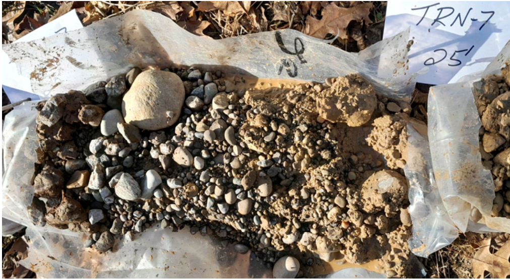
Figure 38. Gravel and sand outwash as encountered in TRN-7 from 20 to 25 ft. bgs.
