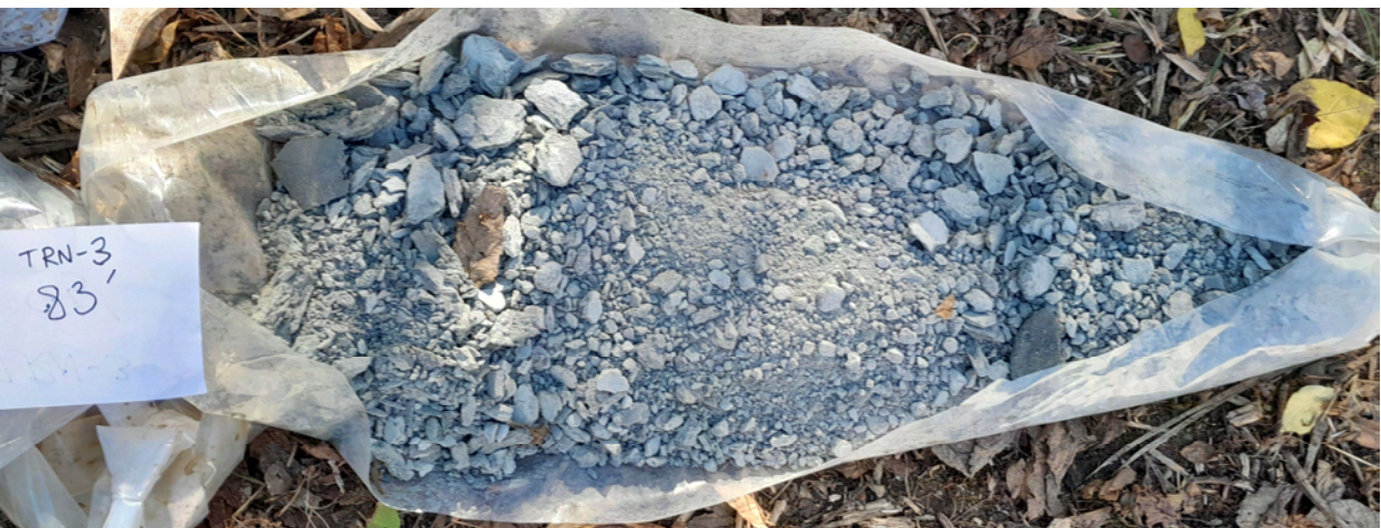
Figure 20. Shale bedrock as encountered from 83 to 85 ft. bgs at TRN-3.
