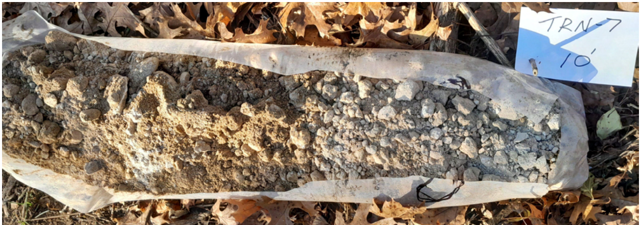
Figure 37. Coarse gravel and cobble outwash (shattered condition) encountered in TRN-7 from 5 to 10 ft. bgs.
