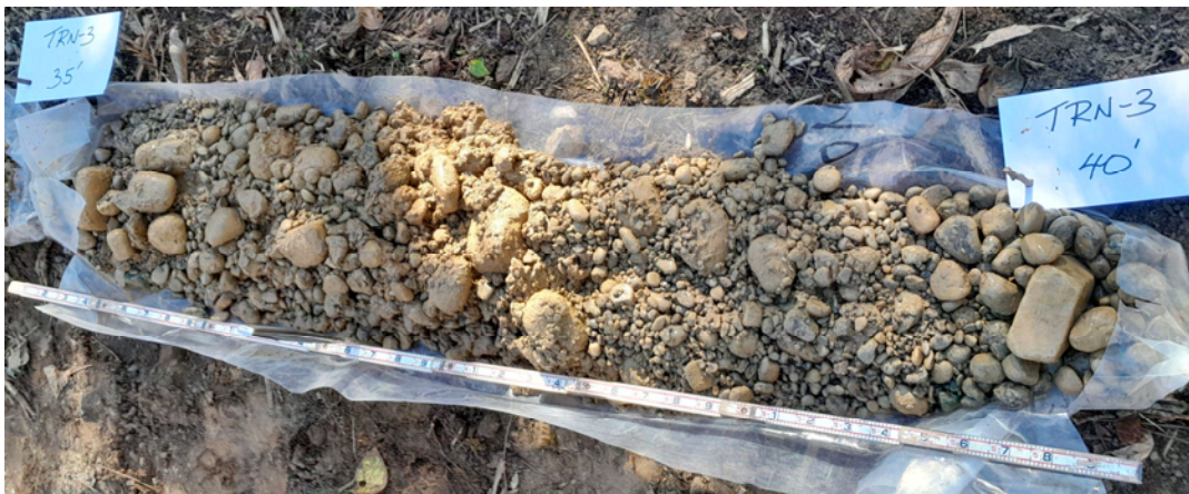
Figure 17. Course outwash gravel & sand of the top of the aquifer in TRN-3 from 35 to 40 ft. bgs.
