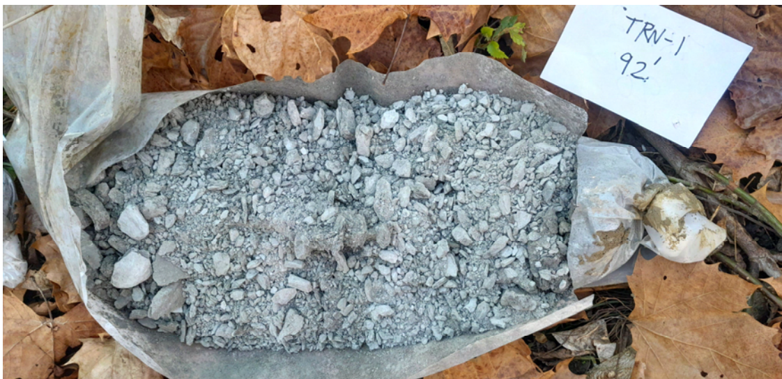
Figure 9. Shale and thin-bedded limestone bedrock as found in TRN-1 from 90 to 92 ft. bgs.
