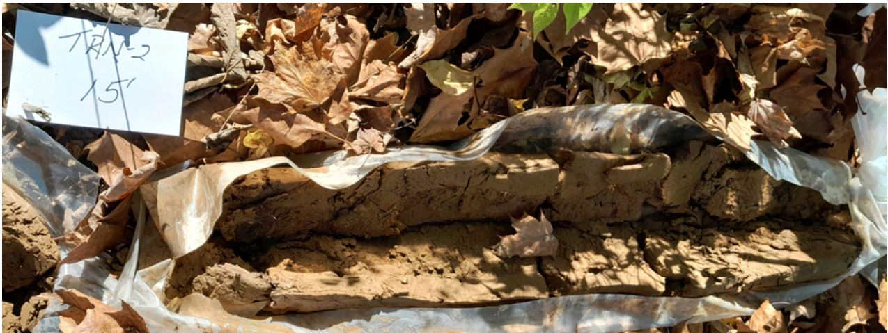
Figure 10. Sandy alluvial deposit as found at TRN-2 from 15 to 19 ft. bgs.
