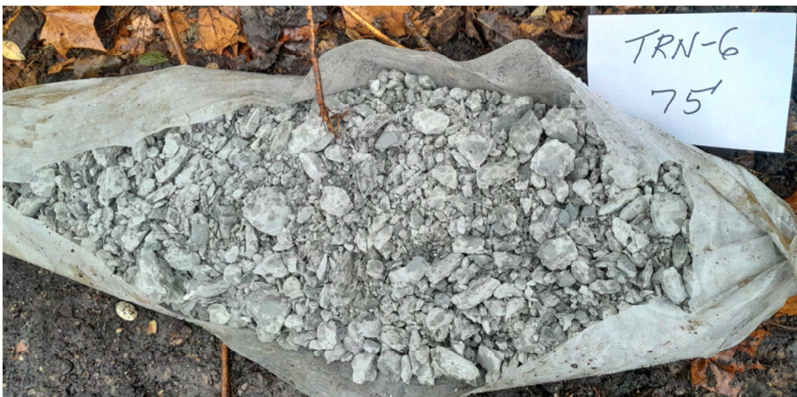
Figure 35. Shale bedrock encountered from 73 to 75 ft. bgs in TRN-6.
