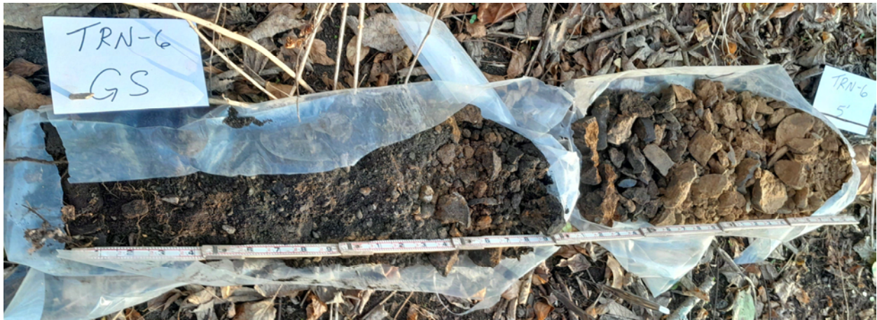
Figure 31. Cinder ash fill soil over brown silty clay soil as encountered from grade to 5 ft. bgs in TRN-6.
