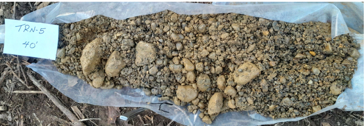
Figure 27. Gravel, sand and cobbles as encountered in TRN-5 from 40 to 45 ft. bgs.
