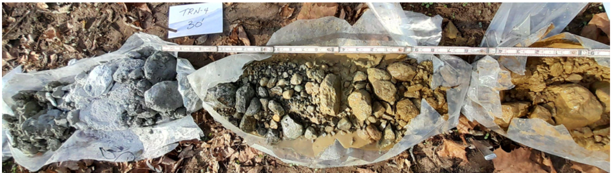
Figure 22. Cobbles and gravel as encountered in TRN-4 from 30 to 35 ft. bgs.
