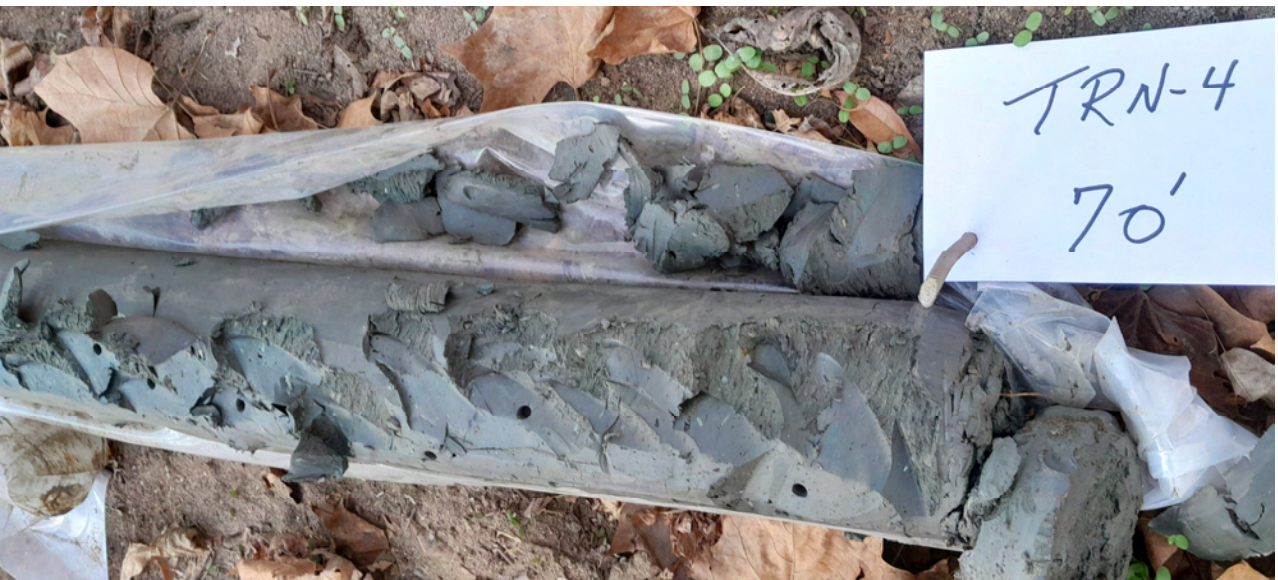
Figure 25. Glacial till deposit the bottom of the BVA encountered from 70 to 77 ft. bgs at TRN-4.
