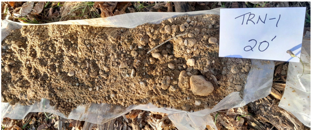
Figure 6. Sample of brown sand and gravel outwash as found in TRN-1 from 15 to 20 ft. bgs.
