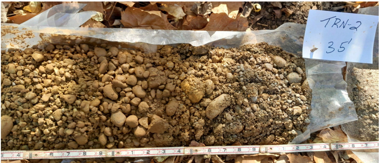
Figure 11. Outwash sand & gravel as found at TRN-2 from 30 to 35 ft. bgs.
