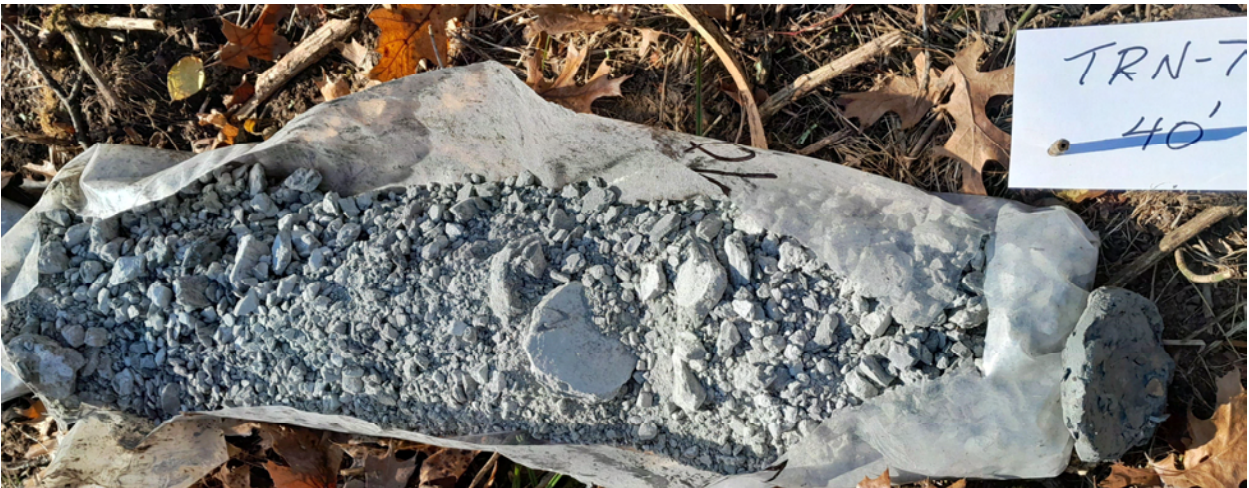
Figure 40. Shale bedrock encountered from 35 to 40 ft. bgs in TRN-7.
