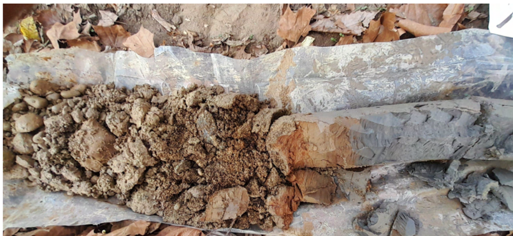
Figure 23. Contact between the outwash aquifer and lacustrine deposit in TRN-4 from 40 to 45 ft. bgs.
