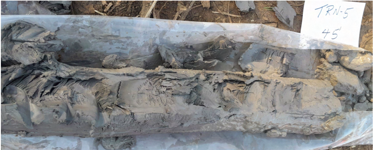
Figure 28. Varved lacustrine clay deposit as encountered from 45 to 58 ft. bgs at TRN-5.
