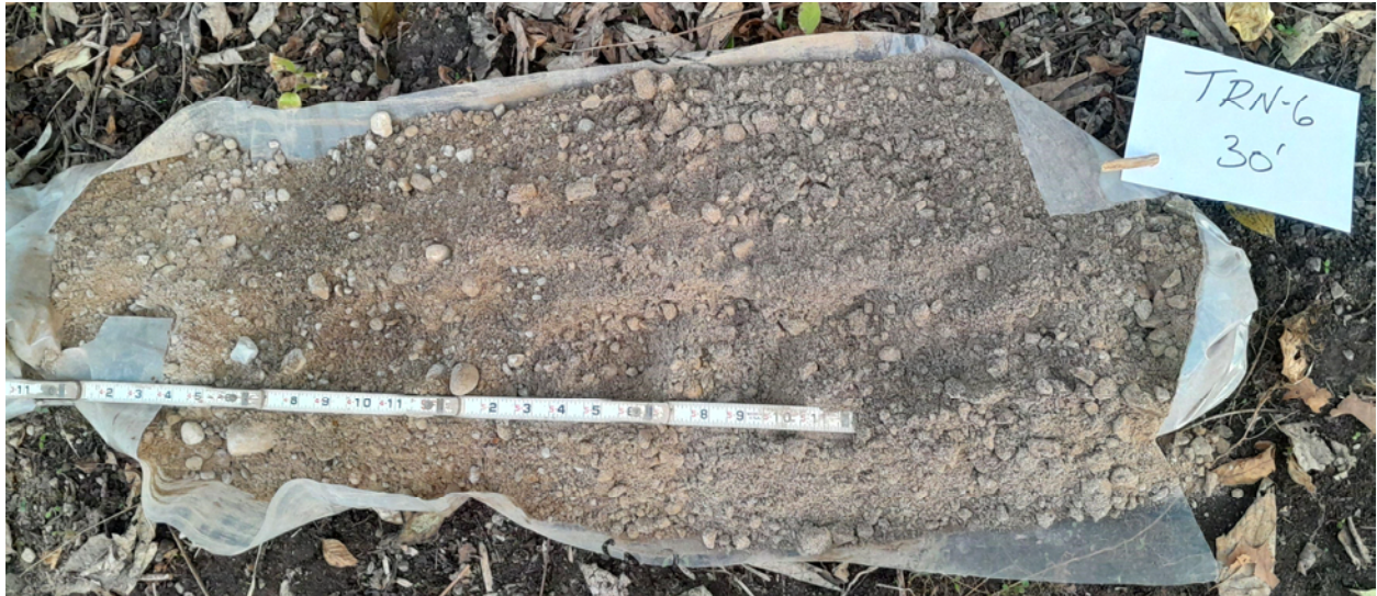
Figure 33. Sand and gravel outwash as encountered in TRN-6 from 25 to 30 ft. bgs.
