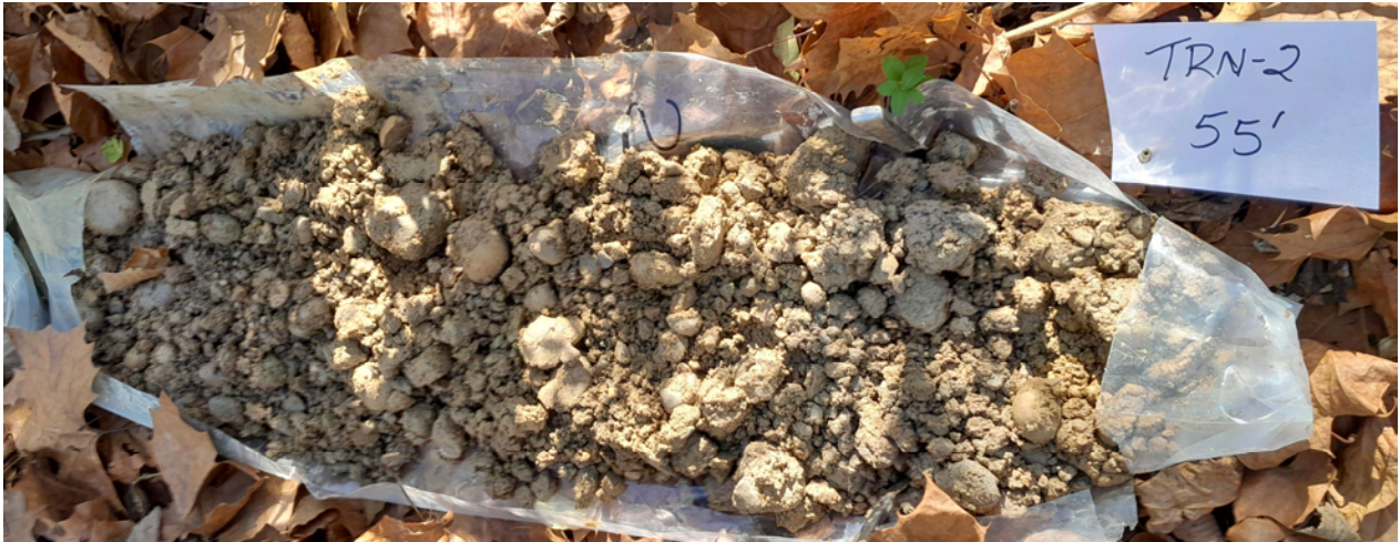
Figure 12. Sample of sand and gravel outwash as found at TRN-2 from 50 to 55 ft. bgs.
