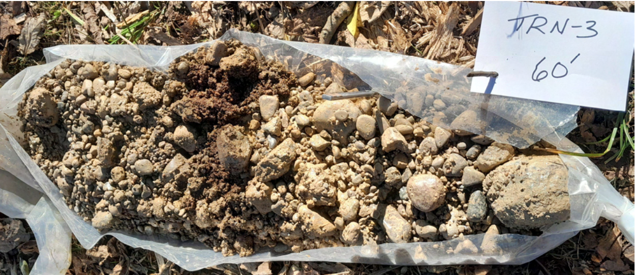
Figure 18. Course outwash gravel in the middle of the aquifer as encountered from 55 to 60 ft. bgs at TRN-3.
