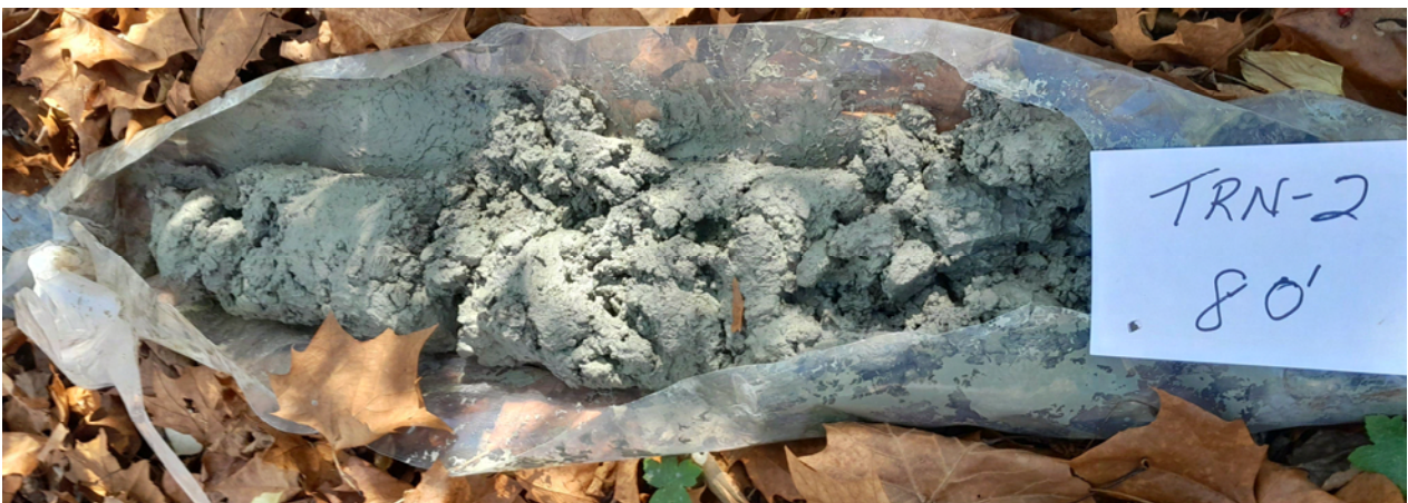
Figure 14. Shale and thin-bedded limestone bedrock as found in TRN-2 from 75 to 80 ft. bgs.
