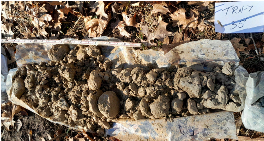
Figure 39. Course clayey sand and gravel outwash encountered from 30 to 35 ft. bgs at TRN-7.
