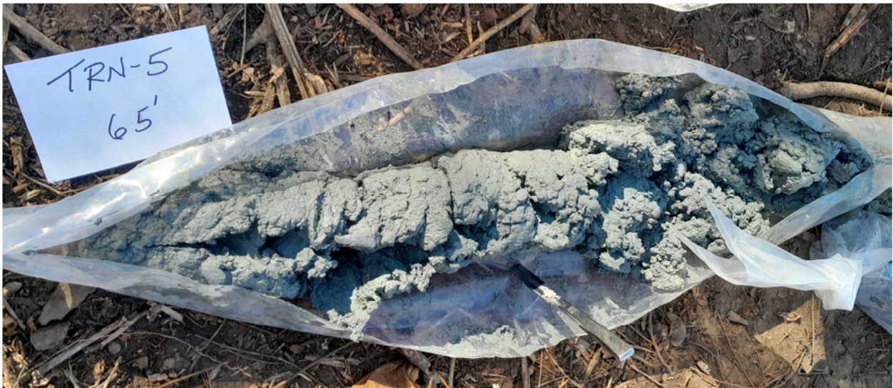
Figure 30. Shale bedrock encountered from 60 to 70 ft. bgs in TRN-5.
